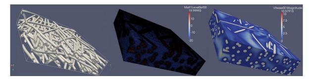
**Figure 2:** Flow on a composite image: iso-value 0 of the phase function  $u_{\varepsilon}$ , mesh and computed velocity-norm
